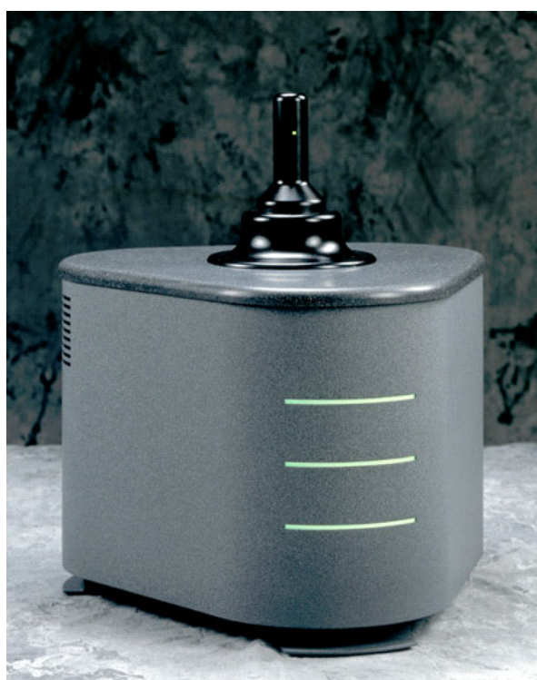
B – CSC Nano ITC III 5300 modelio kalorimetras
